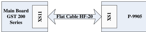
Fig. 1 Connecting with a Control Panel
